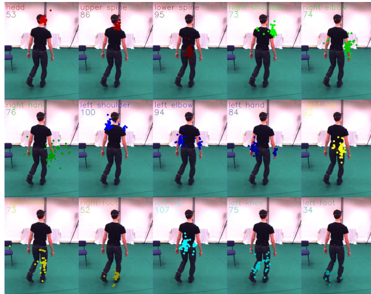
Fig. 2. Body part location ambiguity. For each marker we collect votes casted from visual words. Votes are displayed by small circles. Deciding for an unique location for each marker is not possible at this early stage of pose estimation, since left/right ambiguities cannot be solved just based on identified image structures. Note the left/right ambiguities for nearly all body parts (shoulders, elbows, hands, hips, knees, feet).
